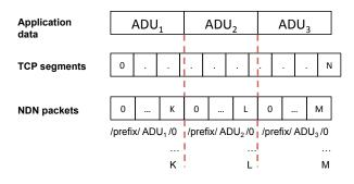
Figure 1: TCP/IP segmentation does not preserve boundaries of application frames (ADUs). NDN segmentation exposes these boundaries through naming.
